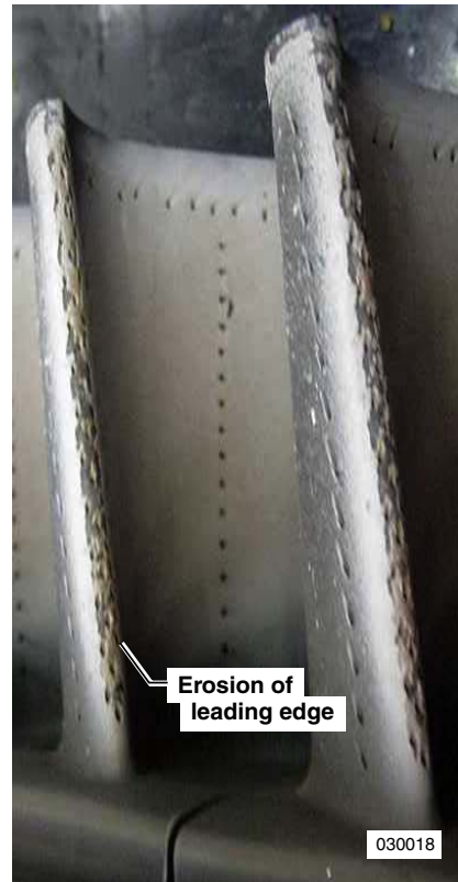
(b) Erosion of leading edge.
