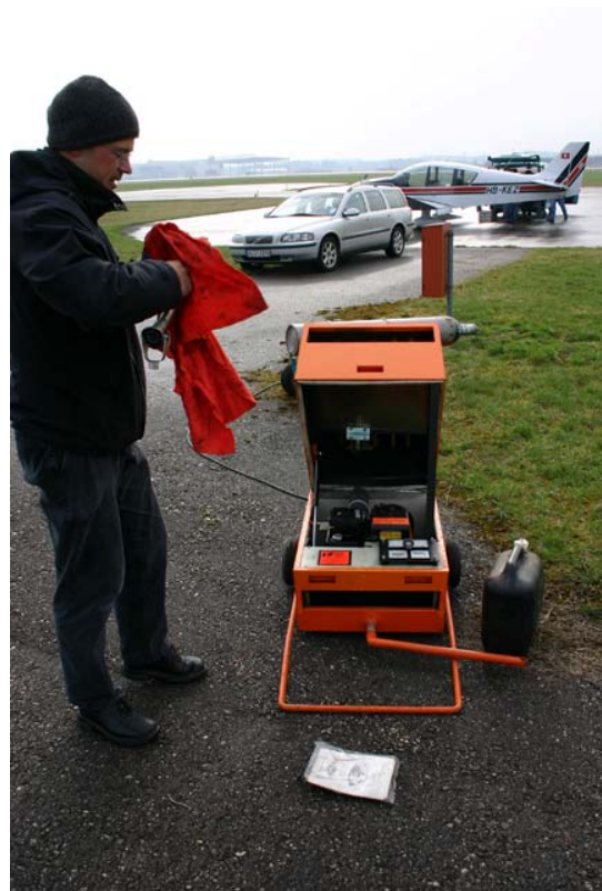
Picture 10: Small ground power unit for In-field supply of electricity.
