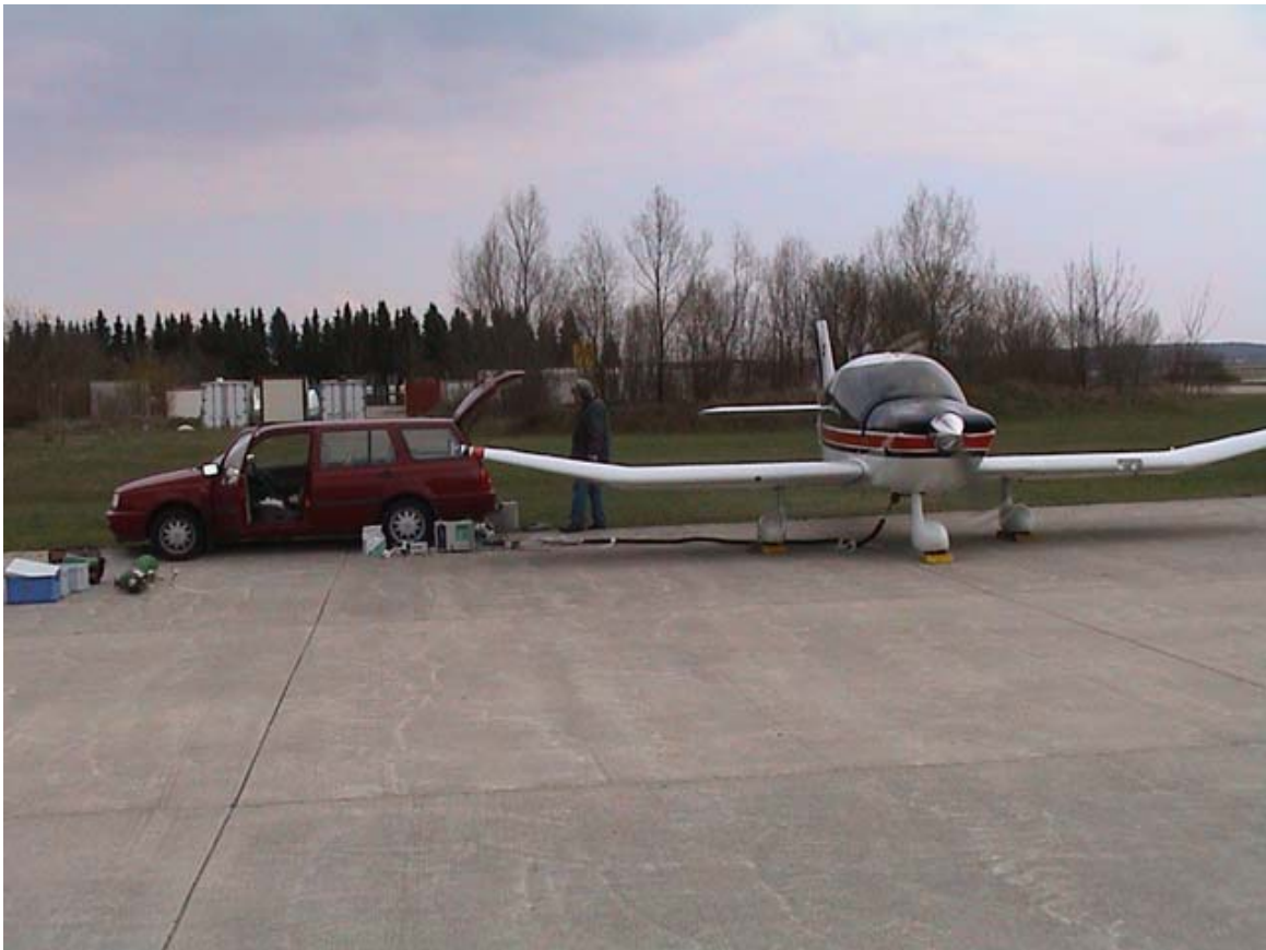
Picture 6: This picture was taken during approach mode measurement. The SMPS is placed in the back compartment of the car (as shown in picture 5) and is brought as nearly as possible to the aircraft, for shortest possible sampling line and lowest possible particle losses.
