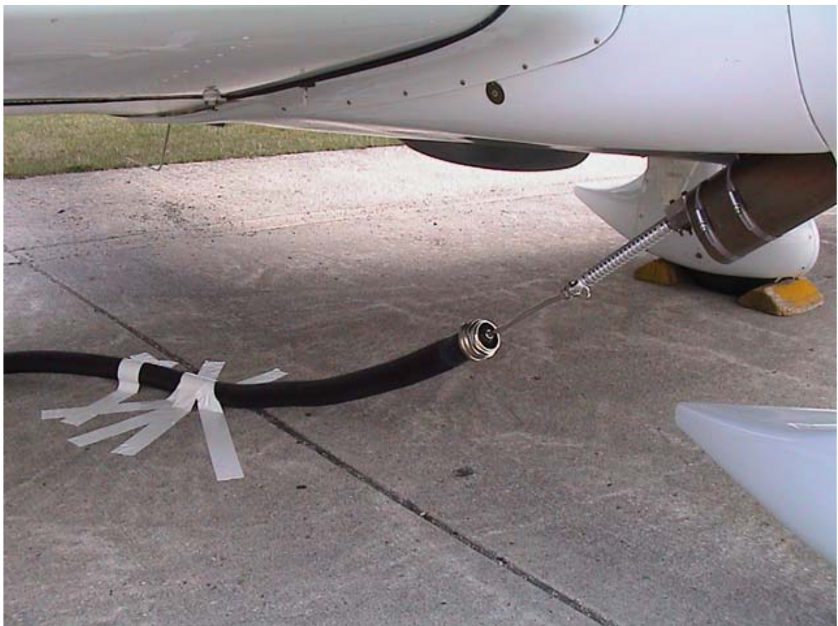
Picture 2: Stainless steel exhaust probe and heated sampling line (150°C). Total length 4.5 meters.
