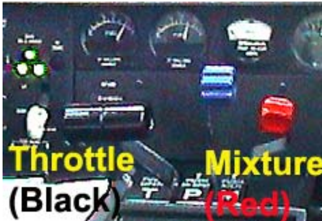
Picture 1: Throttle (black), propeller (blue) and mixture handle (red).
