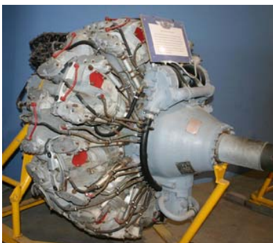
Picture 2: Running lean for thousands of hours is nothing new: The Wright R-3350 engine (DC7 etc.) has been operated on lean mixture during cruise (historical example). As explained above, lean mixture requires better mixture control. In former times this was assured e.g. by symmetrical engine design (equal distances for air intake, symmetrical cooling air flow etc) and a fuel flow and power based leaning technique. A flight engineer was looking after the engines all the time during flight.
