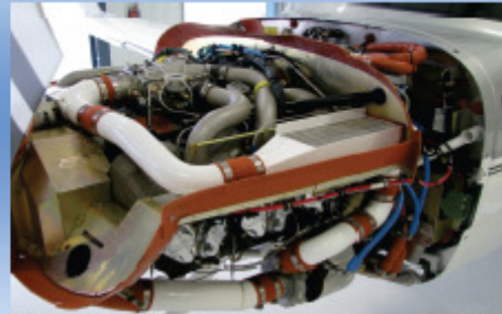
This is a turbo normalizer installation that will not increase power as suggested. This picture is only presented as a way to show an installation.
